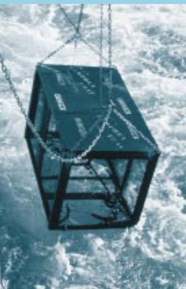
Sea lamprey traps remove spawning lampreys from the system and serve as a source of lampreys for the sterile-male-release-technique.
